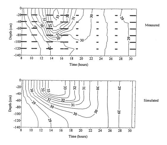
Figure 1 Measured and simulated temperature contours of one of the calibration ponds
